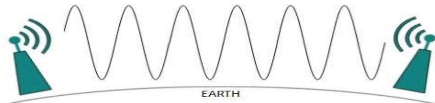
Radio waves of high frequencies are prone to be absorbed by rain and other obstacles. They use Ionosphere of earth atmosphere. High frequency radio waves such as HF and VHF bands are spread upwards. When they reach Ionosphere, they are refracted back to the earth.
