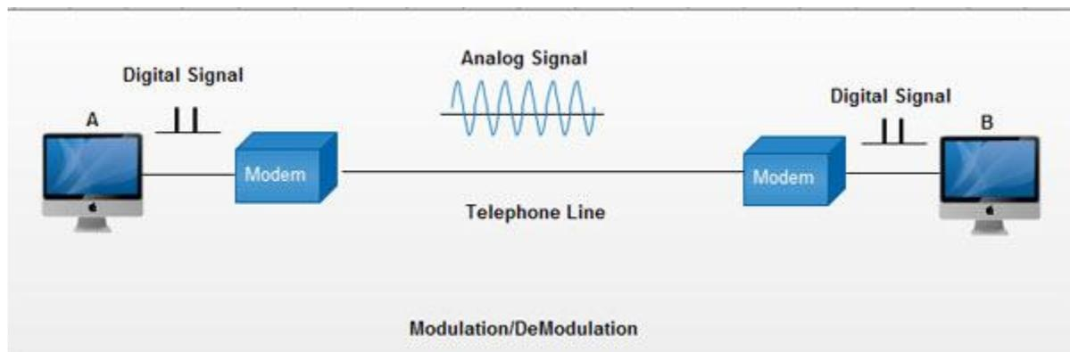
The modem at the transmitting end converts the digital signal generated by DTE into an analog signal by modulating a carrier. This modem at the receiving end demodulates the carrier and hand over the demodulated digital signal to the DTE.
